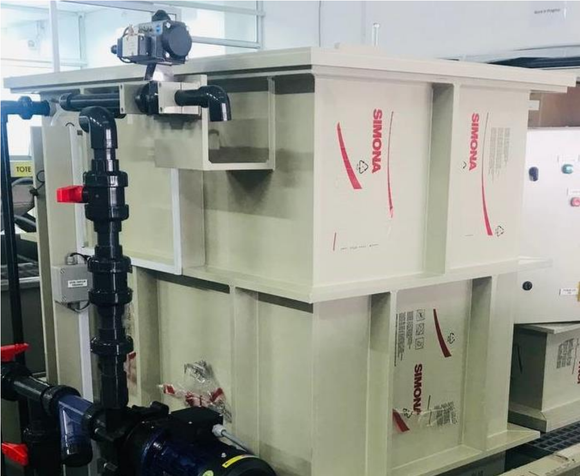
PP TANK FABRICATION
